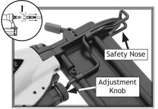
Figure 5. Depth adjustment control.
